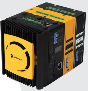
Ultron is a Programmable Logic Controller (PLC) system based on NVIDIA® Jetson that brings high computing power to the edge for industrial applications requiring logic-based decisions for automated processes and machines.
